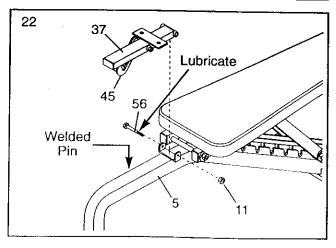
the Sear to the tracker on the Sear Support tube (37) with two M6 x 16mm Screws (3).
